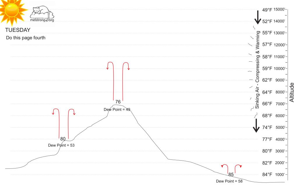
The next day, air is sinking down over New Mexico. This sinking air (called a 'high pressure system') causes the air aloft to warm a bit due to compressional heating. Let's assume that the ground temperature and dew point temperature have not changed from the previous day.
