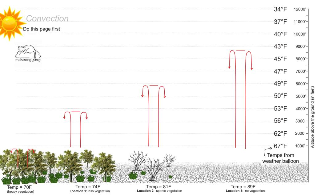
In the above scenario, the sun is shining down on terrain with different amounts and types of vegetation. The ground heats up to the temperatures shown at the surface. A weather balloon is sent up which records the environmental temperatures (shown on the right). The air is perfectly dry with zero humidity - *there will not be any clouds present here.*
